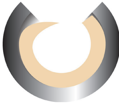
Self-lubricating with teflon liner
