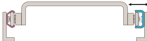
T and U rail allows for misalignment
