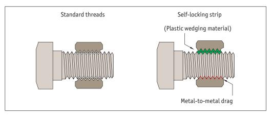
A resilient polymer (generally nylon) strip is inserted into a precisely machined slot that is milled into the thread. The strips are typically positioned one to three threads back from the end of the fastener to assure ease of starting.
